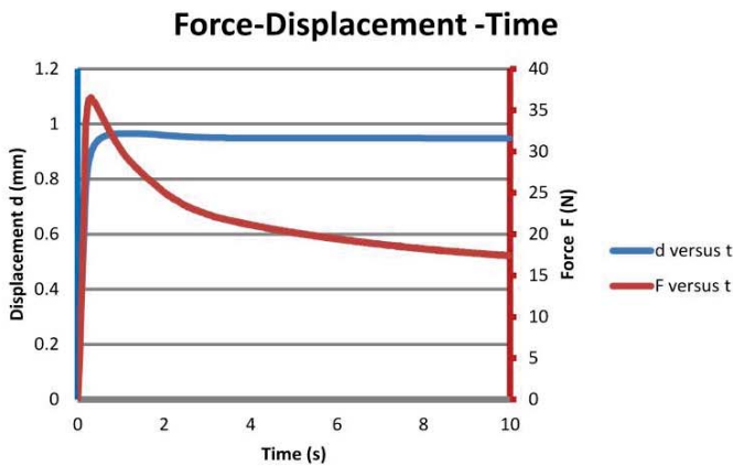
Figure 1a: Applied displacement to the top plate and the force-time response
